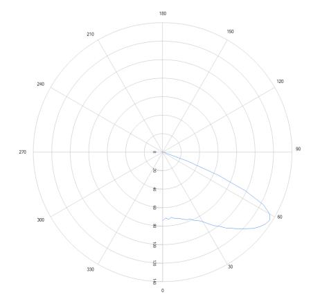
The results for this initial lens produce a peak below  $60^{\circ}$  and more light than desired in the center of the beam. Since we were targeting a  $65^{\circ}$  peak and a higher ratio between the peak and center beam intensity, we will now adjust the lens profile.
